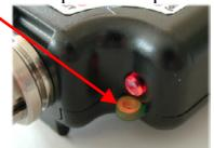
This must be turned on using the USBscope50 software. enabled, the compensation output is a 0 to 3V (approx) square wave with 50% duty cycle and 1KHz frequency. Note that the compensation output will switch off automatically when you close the channel's tab<sup>10</sup>.
